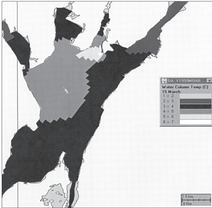
Figure 14. Plan view of daily mean water-column temperature for MOA II hydro-thermal model run on March 15, 1999.
